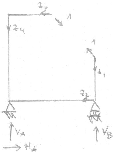
$$\begin{aligned} \rightarrow) & H_A = 0 \\ A) & V_B = 0 \\ \uparrow) & V_A = 0 \end{aligned}$$
