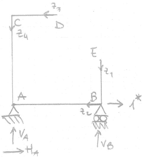
$$\begin{aligned} \rightarrow & H_A = -1 \\ A & \left. \begin{aligned} \uparrow & V_B = 0 \\ \uparrow & V_A = 0 \end{aligned} \right\} \end{aligned}$$
