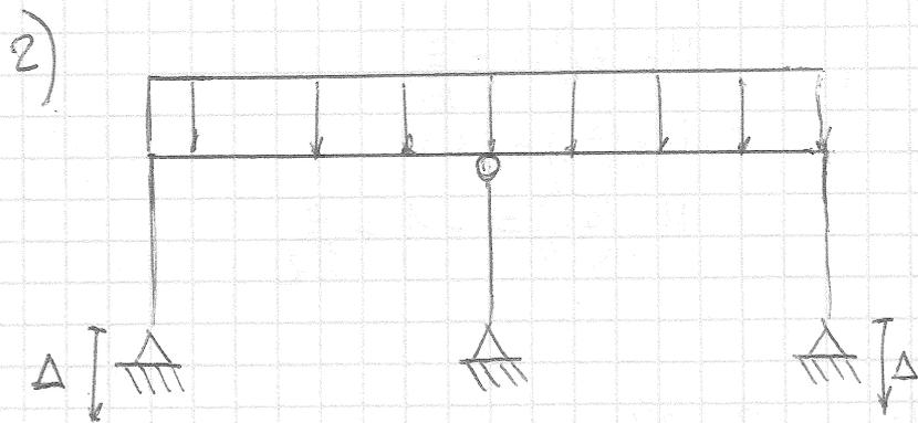
$$\begin{aligned} \Delta &= 1 \text{ cm} = 0,01 \text{ m} \\ J &= 1,943 \cdot 10^{-5} \text{ m}^4 \\ E &= 2,1 \cdot 10^9 \text{ KN/m}^2 \end{aligned}$$
