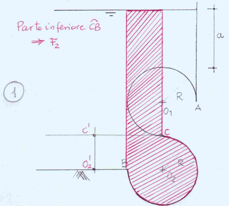
$$(\rightarrow) F_{1x} = \gamma \left( a + R + \frac{R}{2} \right) (LR) = 3.82 \cdot 10^5 \text{ N} = 382 \text{ kN}$$
