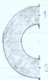
$$x) F_{fx} - p_1 \Omega - p_2 \Omega = \rho \frac{Q^2}{\Omega} + \rho \frac{Q^2}{\Omega}$$
