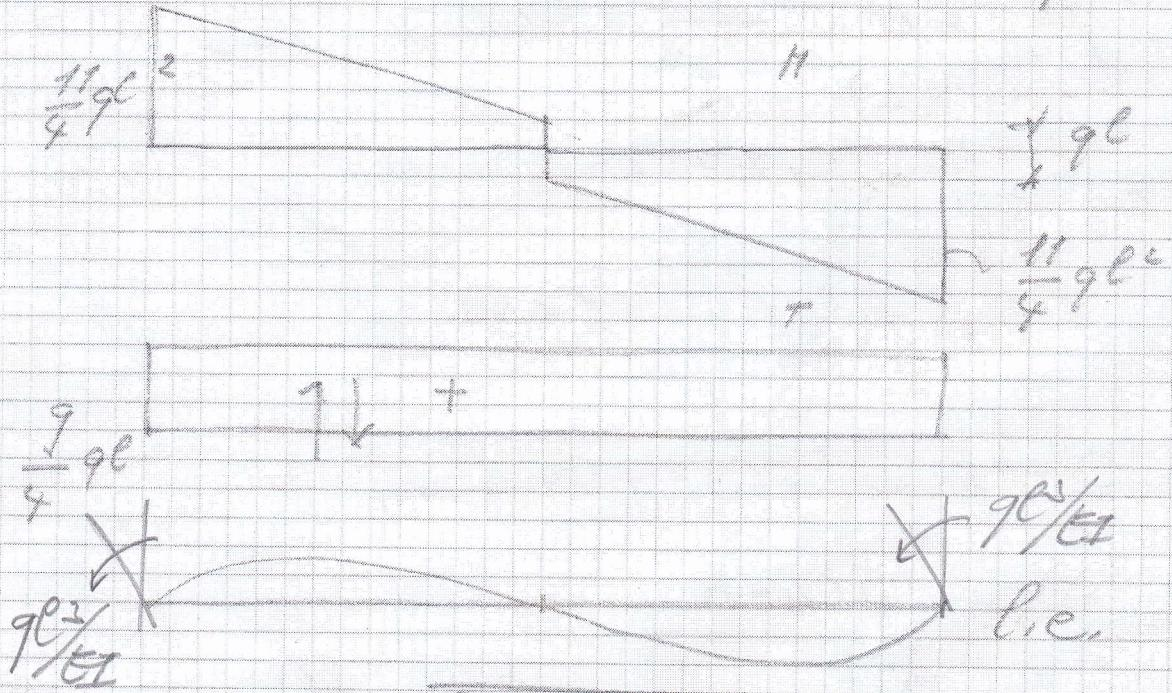
$$\begin{aligned} & \text{At } A \quad \text{at } x=0 \quad M = \bar{q}_A x + \frac{x^2}{2EI} - \frac{ql^3}{4EI} = 0 \\ & \quad \uparrow x \quad \uparrow x^2 \quad x = \frac{q_A}{12EI} \frac{3EI}{x^2} - \frac{\bar{q}_A}{12} \frac{3EI}{l^2} = \\ & \quad = \frac{3}{4}ql - \frac{ql^2}{EI} \frac{3EI}{l^2} = \frac{3}{4}ql - 3ql = -\frac{9}{4}ql \\ & \quad \Rightarrow \quad x = \frac{3}{4}ql \end{aligned}$$
