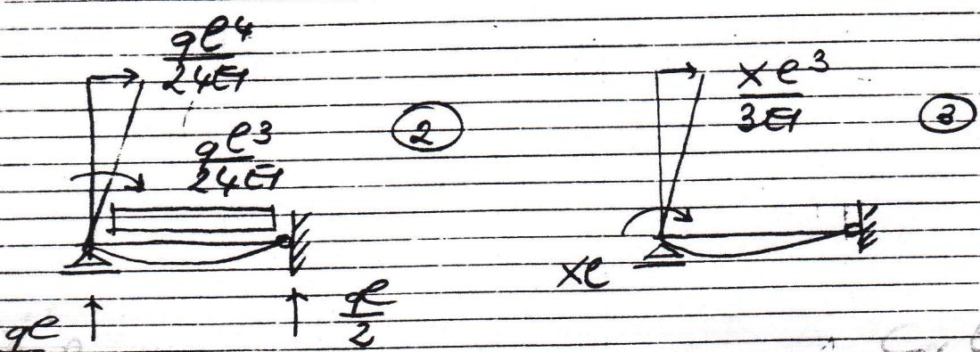
$$\sum \sigma_i = \frac{qe^4}{6EI} + \frac{xe^3}{3EI} + \frac{qe^4}{12EI} + \frac{qe^3}{24EI} + \frac{qe^3}{24EI} + \frac{xe^3}{3EI} - \frac{5qe^4}{24EI} - \frac{xe^3}{24EI} = -x$$
