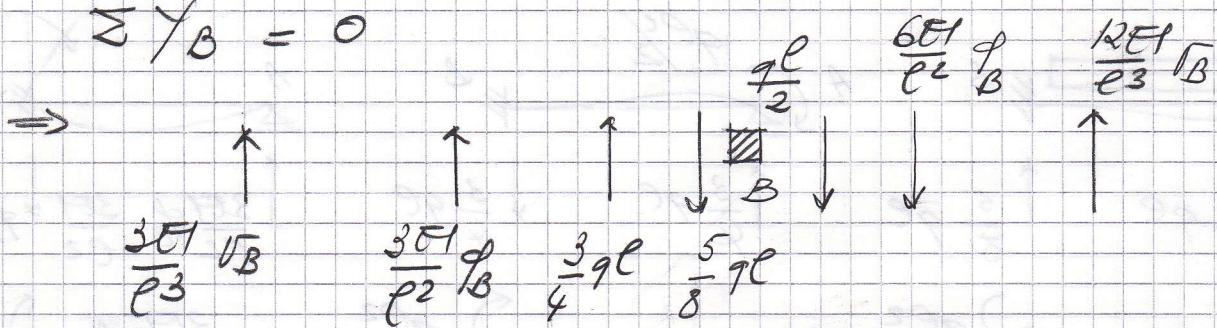
$$\frac{3EI}{l^2} \phi_B - \frac{6EI}{l^2} \phi_B + \frac{3EI}{l^3} \sigma_B + \frac{12EI}{l^3} \sigma_B + \\ + \frac{3qe}{4} - \frac{5qe}{8} - \frac{qe}{2} = 0$$
