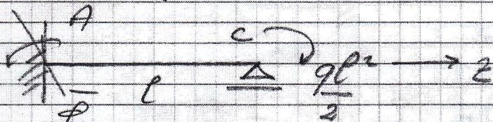
$$P_A \downarrow \quad P_C \rightarrow \quad \Delta \quad \frac{ql^2}{2} \quad \frac{d^4v(z)}{dz^4} = 0 \quad \frac{d^3v(z)}{dz^3} = C_1 = -T(z)/EI$$
