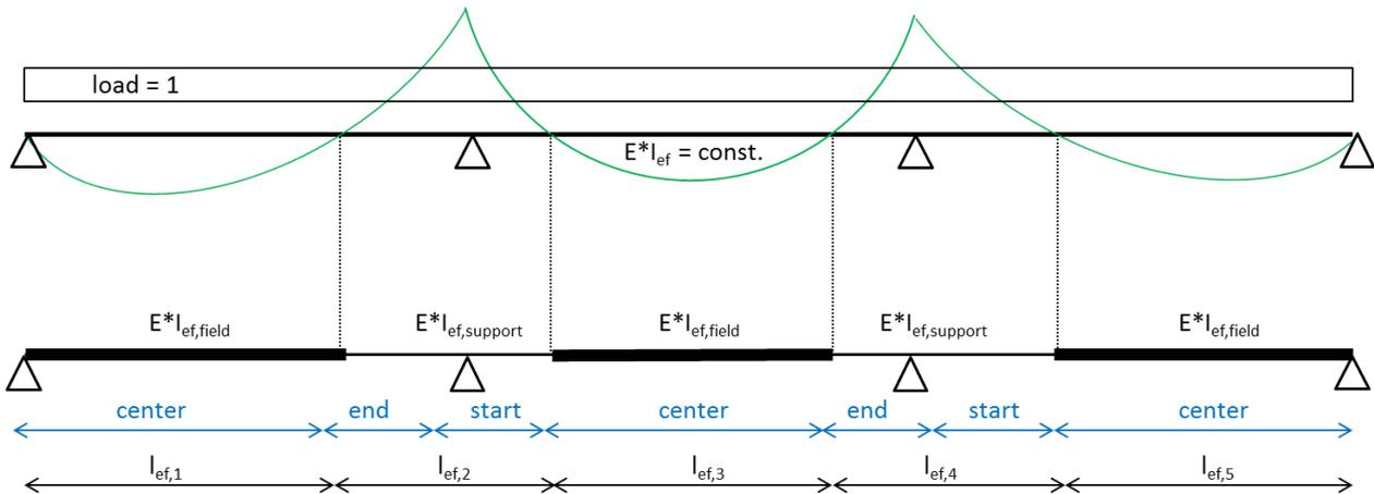
These different  $\gamma$ -values in different parts of a beam are reflected in the design and are indicated in the result:
