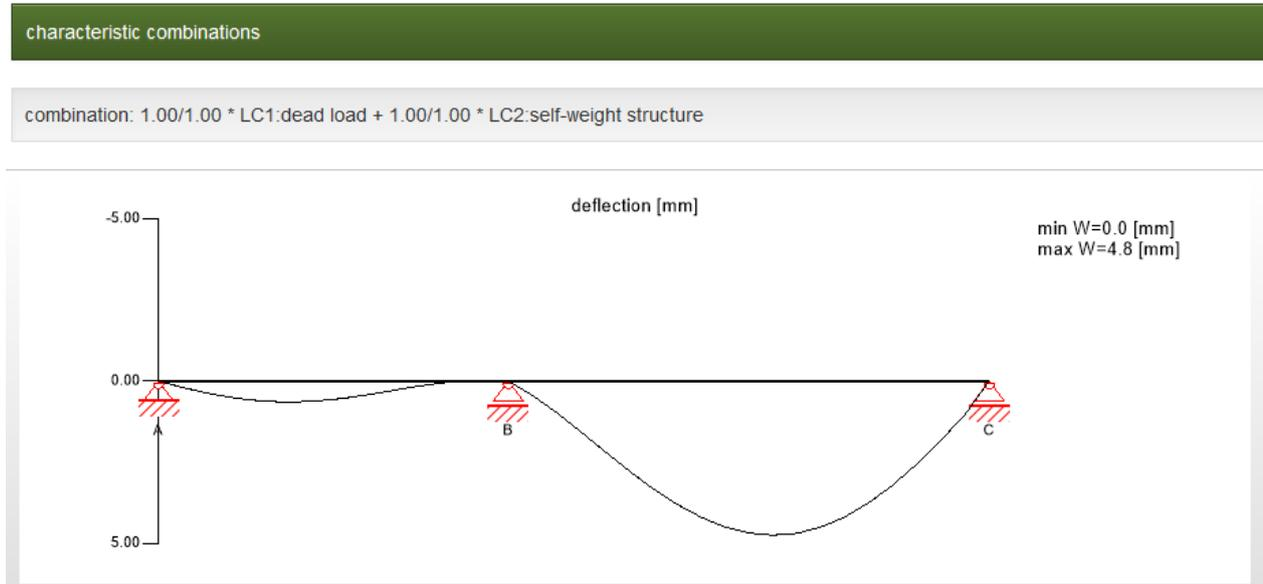
Maximum and minimum values are given next to the curve. Intermediate values are displayed in a table, when clicking the curve.
