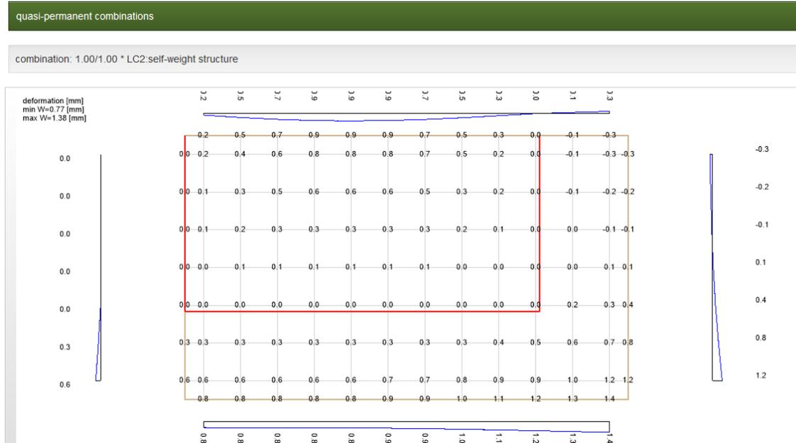
The blue curves to the outside of the panel are the deformation curves of the panel edges.
