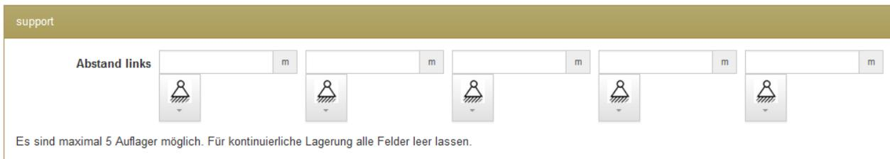
If no data is being entered in this box, then the CLT element will be supported on the entire length of the bottom edge (typical for walls. The linear support in that case is a pin support out of plane ( $M=0$ ). The support will take tension and compression. A non-linear support condition (e.g.: taking compression only, but not tension) is currently not possible in this design tool (possible future development).
