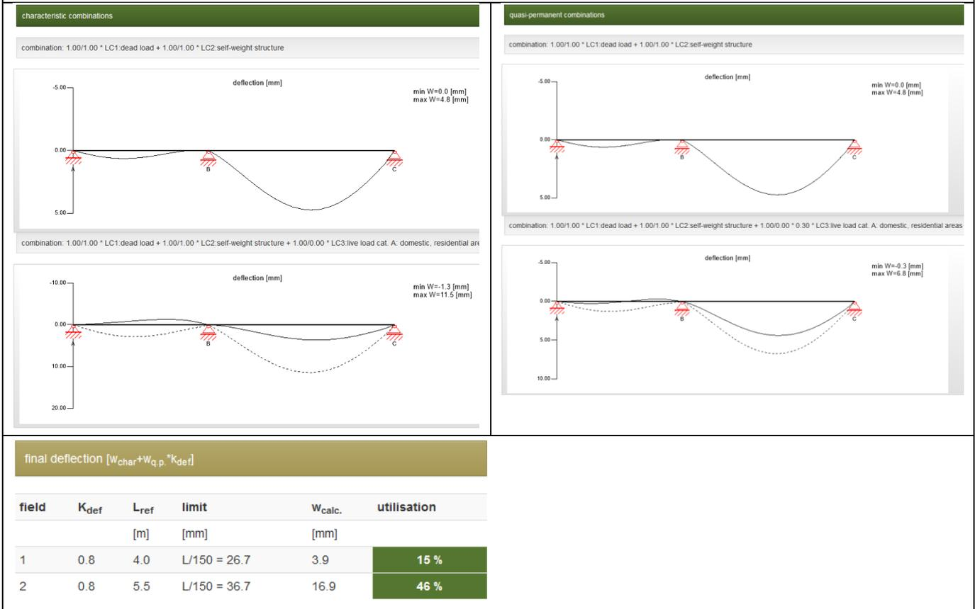
$$W_{fin} = W_{inst} + W_{creep} = \underbrace{11,5}_{\text{characteristic load combination}} + \underbrace{6,8 \cdot \overbrace{0,8}^{k_{def}}}_{\text{quasi permanent load combination}} = 16,94 \text{ mm}$$
