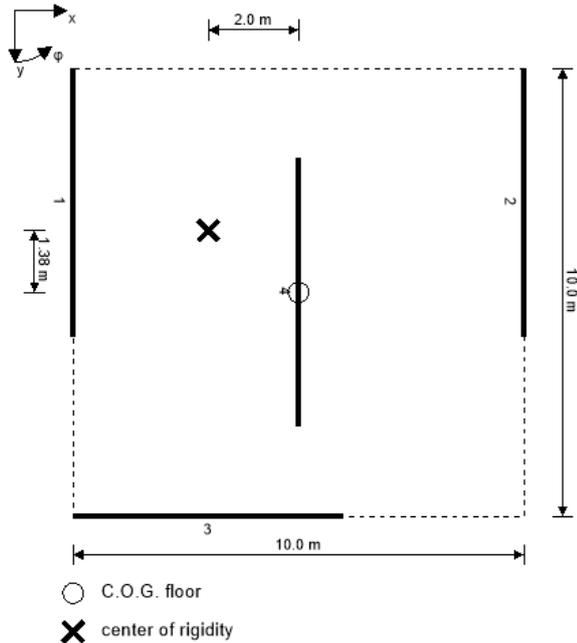
The general results of the RDA module give values of the maximum dimensions, coordinates for C.O.G and center of rigidity, accidental eccentricity, total eccentricity and the stiffness:
