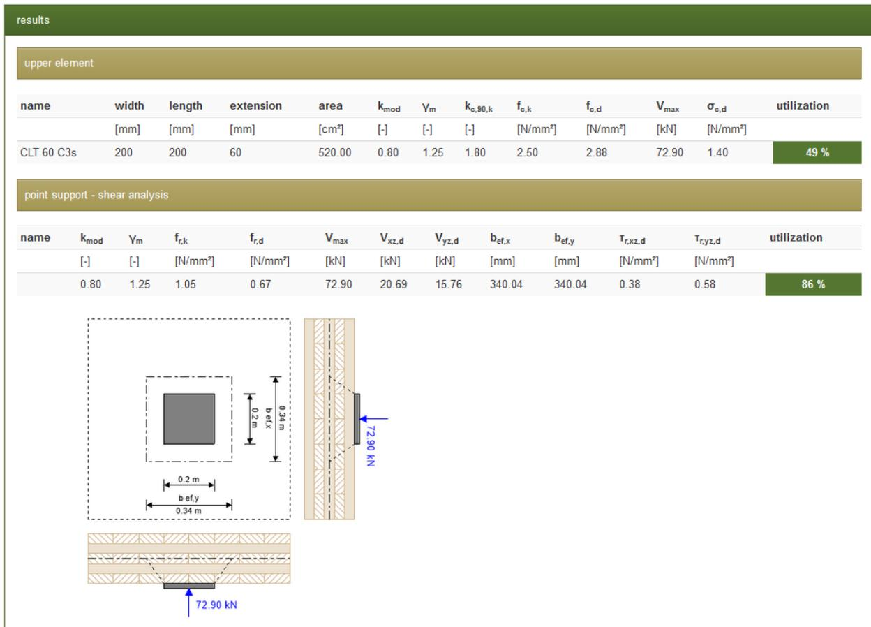
The figure above displays the result of the point support design module, for a central support and delivers results for the bearing pressure perpendicular to the grain and for the rolling shear at the point support.
