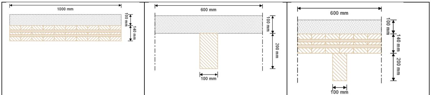
For the case CLT deck with concrete topping above the CLT and ribs below the CLT there are 3 different sub categories, depending on the position of the CLT-deck in relation to the rib:
