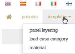
The following templates shall help the user, to pick among common panel layouts, load case categories and materials, that are specific for a given country. By default, some basic data is already included in the templates. The user can add on to the existing template, clicking the “+” icon:
