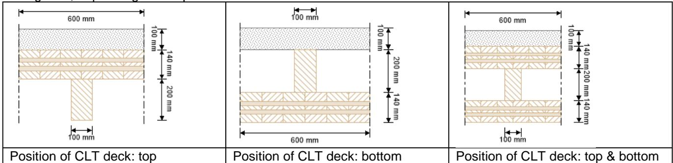
The connection between CLT and the concrete can be assumed rigid (glued, interlocking system, etc.) or flexible (use of mechanical shear connectors).
