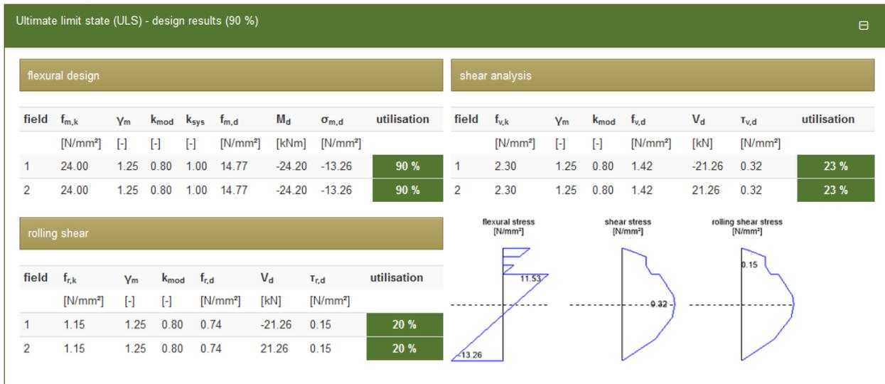
The ULS design results are displayed in a similar way as for the CLT panel design module(see chapter 7.1). The stress diagrams are drawn for the locations within the beam that cause the governing internal forces. If loads in the plane of the rib deck element are entered (see chapter 7.4.3), buckling design will be conducted as well.
