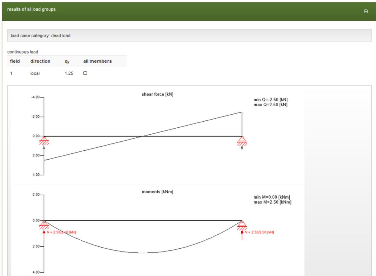
The maximum and minimum values are given in the diagrams. Other values from intermediate points along the beam can be retrieved in a table by clicking the respective curve or diagram:
