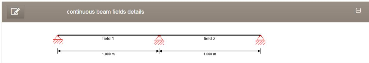
Click edit in order to edit the geometry of the beam. The default system is a beam with 3 supports (2 fields).
