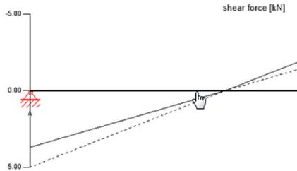
value for 1.35/1.00 \* LC1:dead load + 1.35/1.00 \* LC3:self-weight structure
