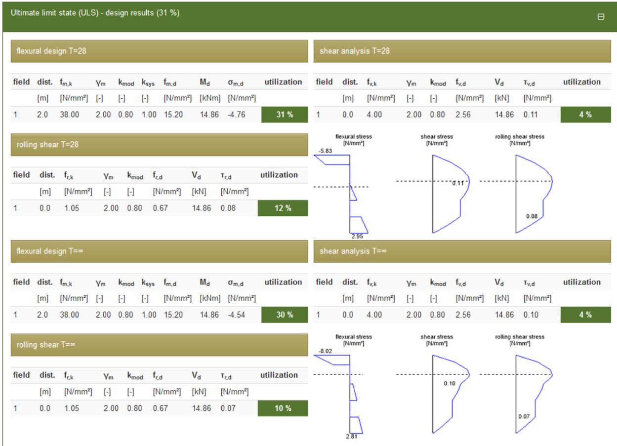
The ULS design results are displayed in a similar way as for the CLT panel design module (see chapter 7.1). The stress diagrams are drawn for the locations within the beam that cause the governing internal forces.
