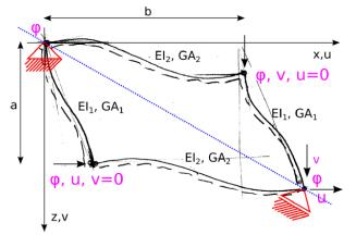
The beam grid model was based on the Bernoulli beam theory with a certain correction coefficient. The global equation matrix for the beam grid model is as follows:
