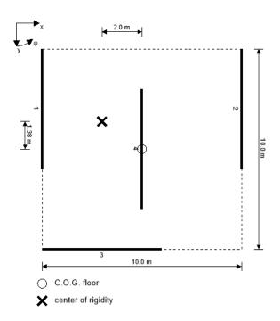
The general results of the RDA module give values of the maximum dimensions, coordinates for C.O.G and center of rigidity, accidental eccentricity, total eccentricity and the stiffness:
