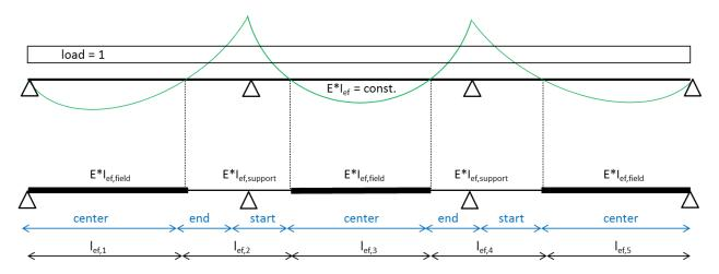
These different  $\gamma$ -values in different parts of a beam are reflected in the design and are indicated in the result:
