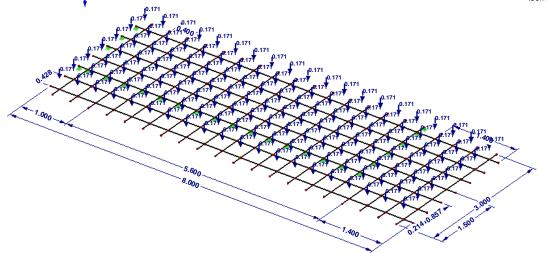
The deformation of the system is being analyzed according to the Timoshenko beam theory, taking all deformation due to flexural moments and shear into account.
