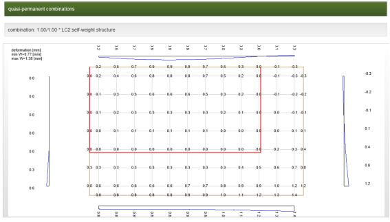
The blue curves to the outside of the panel are the deformation curves of the panel edges.
