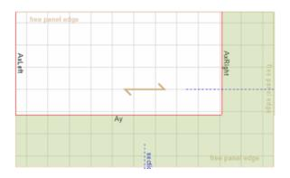
Line load in X direction puts a line load along the panel edge in the cantilever portion on the edge that is oriented in X direction (orange line in figure below):
