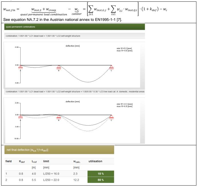
$$w_{net,fin} = \underbrace{w_{inst,2} + w_{creep}}_{quasi \ permanent \ load \ combination} - \underbrace{w_c}_{camber} = \underbrace{\left[\sum_{j \ge 1} w_{inst,G,j} + \sum_{i \ge 1} \psi_{2,i} \cdot w_{inst,Q,i}\right]}_{6.8 \ mm} \cdot \left(1 + \underbrace{k_{def}}_{0,8}\right) - \underbrace{w_c}_{0} = 12,24 \ mm$$
