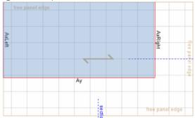
Surface loads on the exterior part of the panel (area that is on the other side of the supports – colored green in the figure below)
