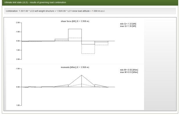
The design governing shear force and moments are displayed in the diagrams. All internal forces are being calculated at the intersection points of the beam grid model. That is the reason, why the curves are not smooth, but polygonal. The values are given for a beam grid element with a given width (= mesh width of the beam grid model). The exact width of the beam elements is given in the section properties, in the result page:
