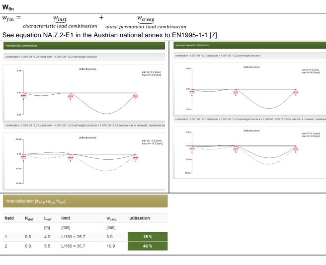
$w_{fin} = w_{inst} + w_{creep} = \underbrace{\underbrace{11,5}}_{characteristic \ load \ combination} + \underbrace{\underbrace{6,8 \cdot \widetilde{0,8}}_{quasi \ permanent \ load \ combination}}^{k_{def}} = 16,94 \ mm$
