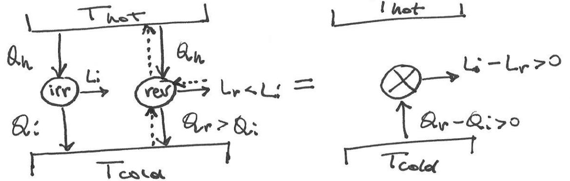
$$\eta_{car} = \eta_{rev} = \eta_{+}(T_{hot}, T_{cold}) = 1 - \left(\frac{Q_{cold}}{Q_{hot}}\right)_{rev} = 1 - \frac{T_{cold}}{T_{hot}} = \eta_{max} \left\{ \begin{array}{l} \text{cfr. kelvin} \\ \left(\frac{Q_{cold}}{Q_{hot}}\right)_{rev} = \frac{T_{cold}}{T_{hot}} \end{array} \right.$$
