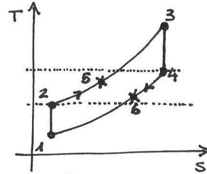
$$\epsilon = \frac{q_{rif}}{q_{rif,max}} = \frac{h_5 - h_2}{h_4 - h_2} \approx \frac{T_5 - T_2}{T_4 - T_2}$$
