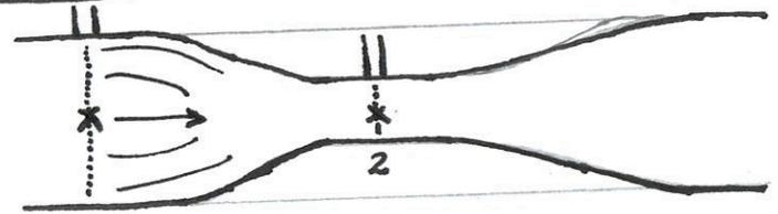
$$z_1 + \frac{P_1}{\rho g} + \frac{v_1^2}{2g} = z_2 + \frac{P_2}{\rho g} + \frac{v_2^2}{2g} \quad ; \quad Q_v = vA = v \frac{\pi D^2}{4}$$
