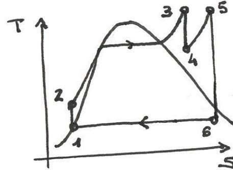
$$q_{cl} = q_{23} + q_{45} = (h_3 - h_2) + (h_5 - h_4)$$
