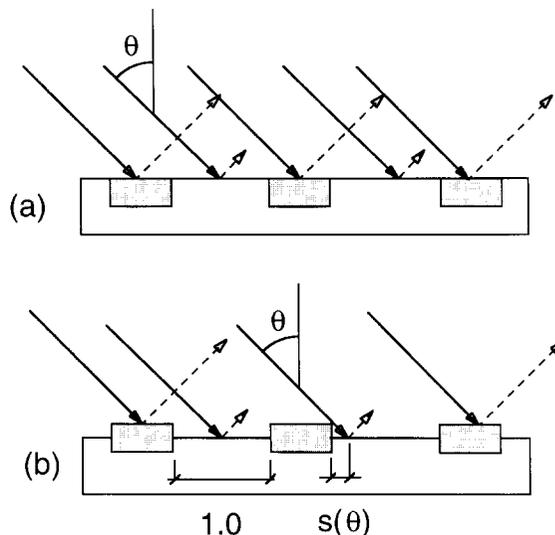
Fig. 4. Diagrams showing the simplified surface of an unencapsulated solar cell: (a) the light is reflected by the surface from the fingers and from the 'optically active' area of the semiconductor; and (b) in a real unencapsulated cell, the fingers protrude above the cell surface and produce a shadowing effect over the active area.
