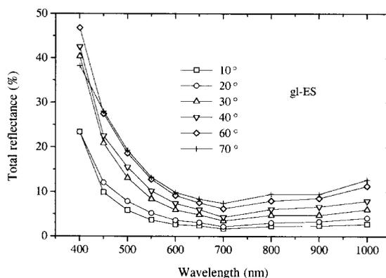
Fig. 13. Filter spectral reflectance,  $R_{\text{tot}}(\theta, \lambda)$ , of the 'gridless' ES (EuroSolar) cell, at different incidence angles. The optical loss increases quite homogeneously on the entire spectrum, at increased incidence angles. At short wavelengths, the reflectance reaches values as high as about 50%.
