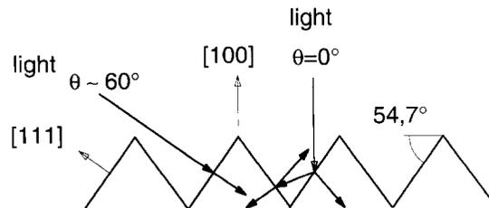
Fig. 7. Schematics of the geometric optics describing the reflection of a light beam on the surface of a silicon sample textured by regular pyramids. Both low and high angles of incidence are favoured by this type of surface texturization.
