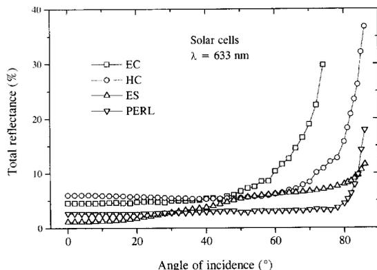
Fig. 6. Curves of total reflectance,  $R_{\text{tot}}(\theta)$ , of four types of tested solar cells, as a function of the incidence angle of the laser beam. The irradiance on the sample was about  $1 \text{ W/cm}^2$ , at  $\theta = 0^\circ$ . All the textured cells show superior optical properties. The PERL cell, in particular, shows the lowest reflection, that maintains up to an angle as high as  $80^\circ$ .
