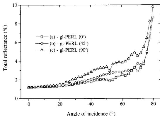
Fig. 10. Total reflectance,  $R_{\text{tot}}(\theta)$ , at  $\lambda = 633$  nm, of the 'gridless' PERL cell at different azimuth angles of the incident laser beam. The difference between  $\phi = 0^\circ$  and  $\phi = 90^\circ$  is attributed to nonsymmetrical photolithography and wet etching process.
