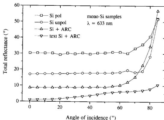
Fig. 5. Total reflectance,  $R_{\text{tot}}(\theta)$ , of mono-silicon samples with different surface treatments. The reflectance is shown as a function of the incidence angle of a 1 mW He–Ne laser beam of  $\lambda = 633 \text{ nm}$ . The irradiance at  $\theta = 0^\circ$  was about  $50 \text{ mW/cm}^2$ . The textured and ARC coated silicon shows the lowest reflectance even at the highest angles.
