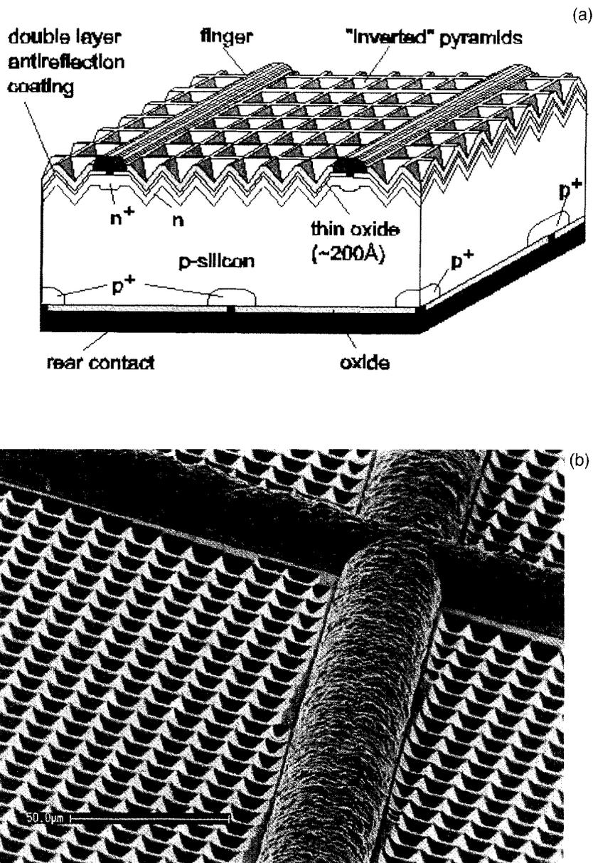
Fig. 2. (a) The structure of the PERL cell. The cell front surface, processed by photolithography, is textured with regular pyramids. In the figure, the pyramids have bases parallel to the fingers. (b) SEM picture of the PERL cell surface, with the semi-circularly shaped fingers and the inverted pyramids. The pyramids form an array which is slightly inclined with respect to the fingers. The segment in the figure is equivalent to  $50 \mu\text{m}$ .
