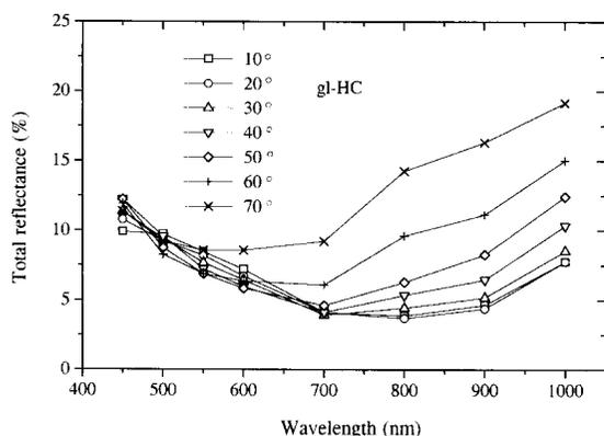
Fig. 12. Filter spectral reflectance,  $R_{\text{tot}}(\theta, \lambda)$ , of the 'gridless' HC (honeycomb) cell, reported at different incidence angles. The optical loss of the cell is particularly evident at long wavelengths. At short wavelengths, the cell reflectance becomes quite insensitive to the incidence angle. At some angles, the optical loss becomes even reduced.
