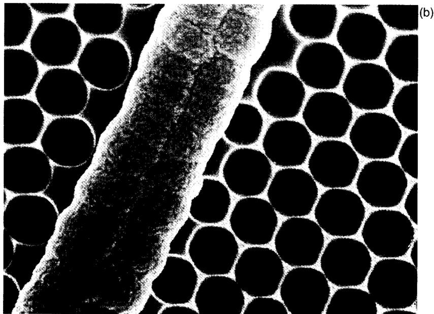
Fig. 3. (a) The structure of the 'honeycomb' (HC) cell. The HC cells have a surface structure consisting of hexagonally placed hemispherical 'wells'. They were processed similarly to the PERL cells, except for their thinner multicrystalline substrate and for the surface texturization. (b) SEM picture of the HC cell surface, with the hemispherical wells. The fingers are similar to those of the PERL cells.
