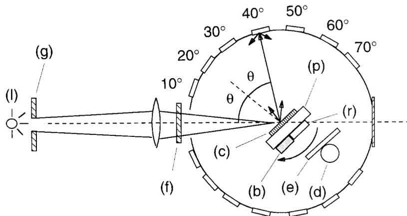
Fig. 1. Schematic diagram of the top view of the ROSE apparatus in the configuration for filter spectral reflectance measurements on small sample. The sample is placed at the center of the sphere. All the ports, except  $0^\circ$  for the input of light, are closed. A  $40^\circ$  total reflectance measurement is illustrated.
