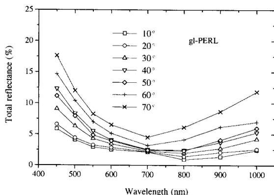
Fig. 11. Filter spectral reflectance,  $R_{\text{tot}}(\theta, \lambda)$ , of the 'gridless' PERL cell, reported at different incidence angles of a QTH lamp light beam. The irradiance at  $\theta = 0^\circ$  incidence was about  $1 \text{ mW/cm}^2$ . The increasing of  $\theta$  increases the selectivity of the cell for the collection of light at intermediate wavelengths.
